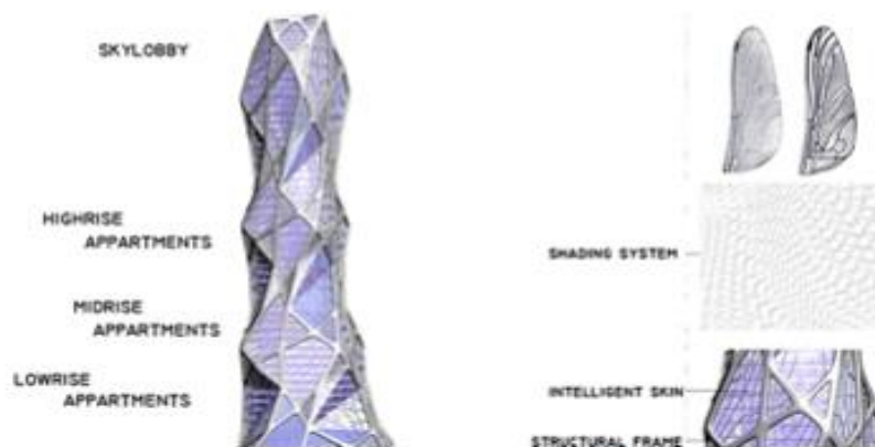
Fig. 5. Lava bionic tower intelligent system [44].
