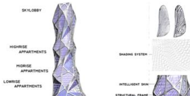
Fig. 5. Lava bionic tower intelligent system [44].
